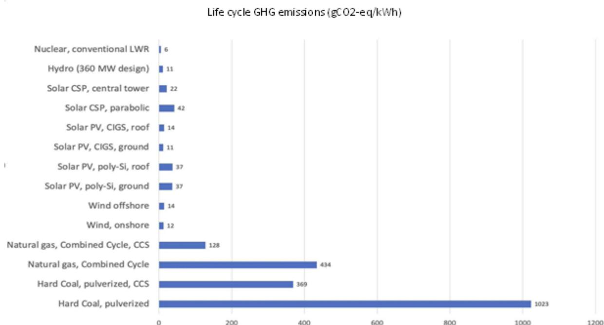
**Figure 5.** Life cycle greenhouse gas emissions intensity of various electricity generation methods.
